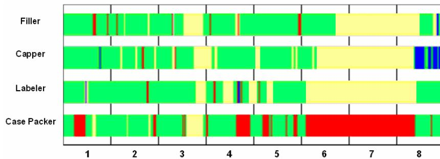
In this example, a particular filling line was exhibiting poor performance and resulting in OEE of 60.57%. The Acumence line flow analysis tool shown above was used to visualize the operating state of each machine on the line during a shift. The Case Packer was identified as a significant bottleneck in the process with downtime being identified as the contributing factor.
